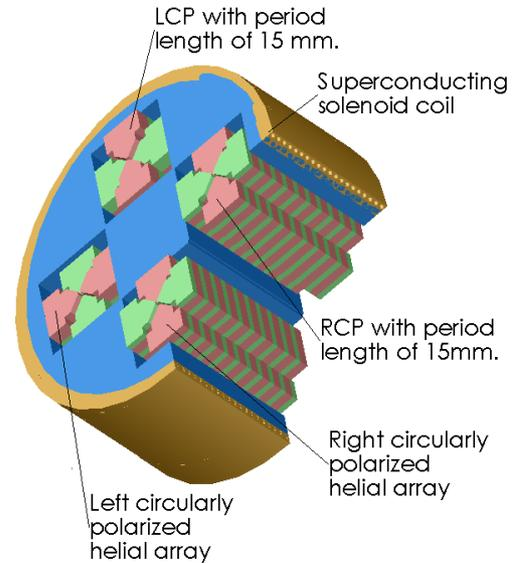
Fig. 6 The configuration of revolving multi-magnetic arrays.
