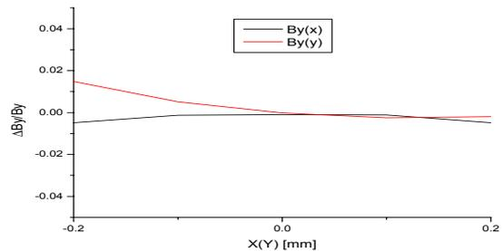
Fig. 4 The vertical field distributions along the horizontal axis at  $y=0 \text{ mm}$  and the vertical axis at  $x=0 \text{ mm}$ .
