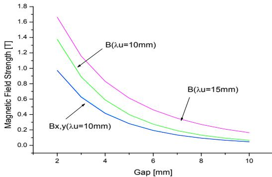
Fig. 2 The variation of the peak fields as a function of the magnetic gap at a current density of  $30 \text{ A/mm}^2$ .
