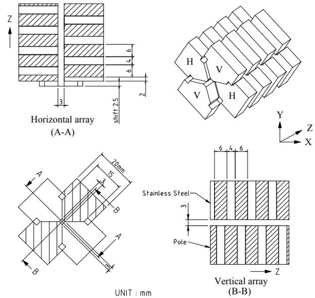
Fig. 1 Schematic view of the helical staggered array
