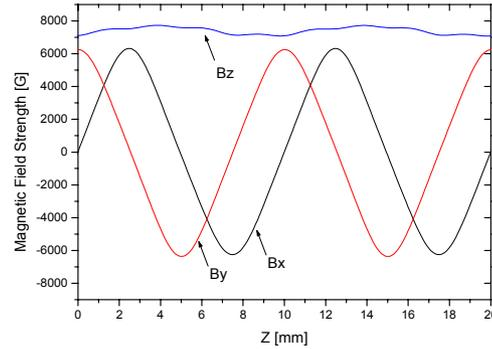
Fig. 3 The horizontal and vertical fields in a 10-mm period length, derived from solenoid field
