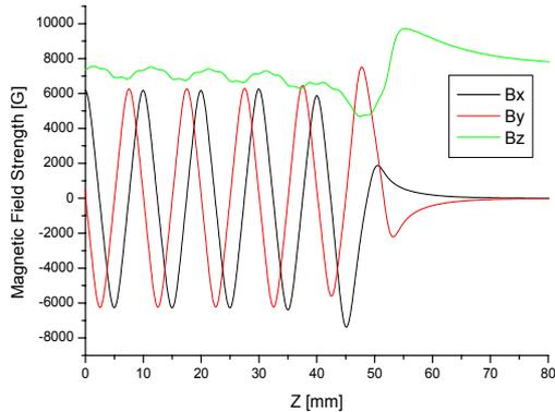
Fig. 5 The calculated vertical, horizontal and longitudinal field distributions at the end pole region.
