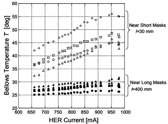
Figure 4: Behaviour of bellows temperature,  $T$ , against HER beam current.
