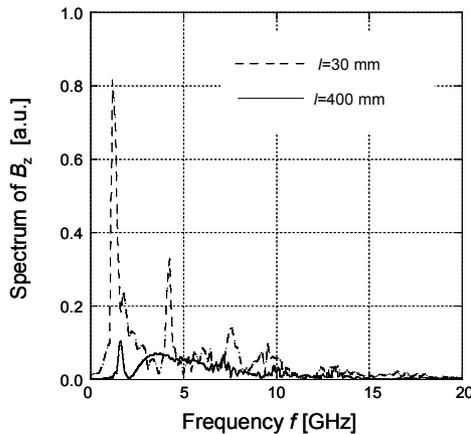
Fig. 5: Spectrum of  $B_z$  for the new long mask ( $l = 400 \text{ mm}$ ) and the previous short mask ( $l = 30 \text{ mm}$ ).
