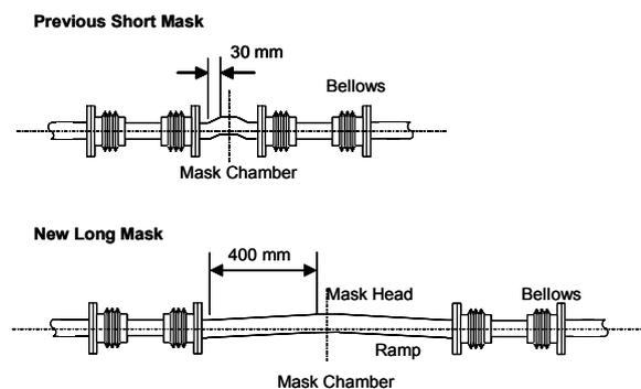
Figure 1: Previous short mask and new long mask. The length of the ramps was expanded from 30 mm to 400 mm.
