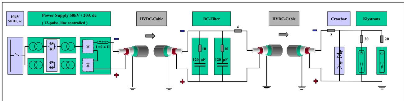
Figure 8: DESY II – Installation consisting of 3 sections (Power Supply, RC-Filter and Klystron Hall)
