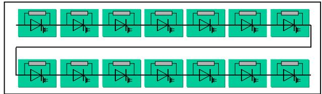
Figure 2: Electrical configuration of the LTT crowbar
