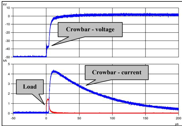
Figure 5: Crowbar operation at nominal voltage
