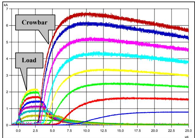
Figure 4: Crowbar operation at different operating voltages (Parameter  $U_{dc} = 10 / 20 / 30 / 40 / 50 / 60 / 70 / 76$  kV)
