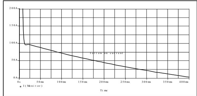
Figure 7: Simulation of the so-called follow through-current introduced by the power-supply smoothing choke.
