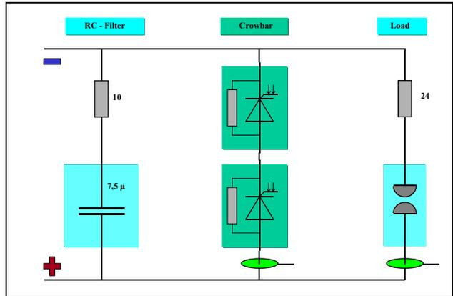
Figure 3: Test set-up
