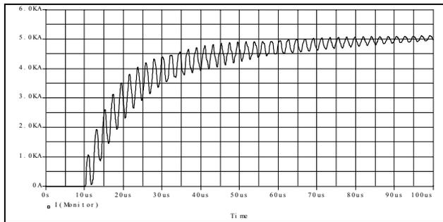
Figure 6: Simulation of the starting edge of the Crowbar current under no-load discharge conditions.
