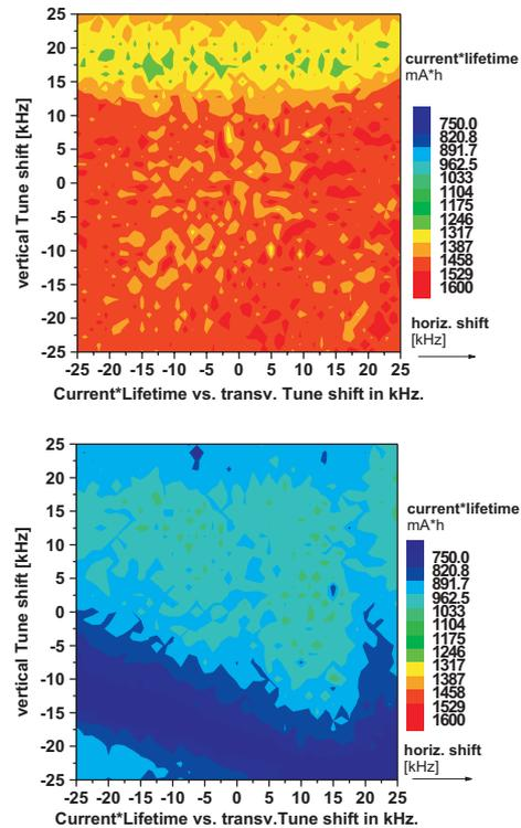
Figure 1: Tune scans with ID UE56 open (above) and closed to 16.6 mm (below). Parameter shown in colour code is current  $\times$  lifetime in mA\*h. Center points mark the actual working point at  $f_x=1060$ kHz  $f_z=925$  kHz (17.848/6.74). BESSY II revolution frequency is 1249 kHz.
