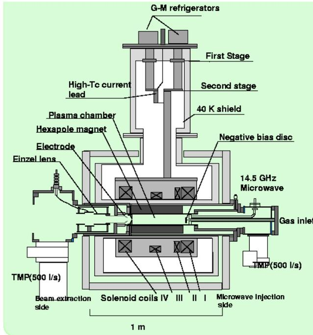
Figure 2: The RAMSES 18 GHz ECR ion source.
