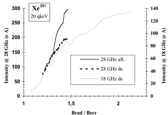
Figure 2 : Effect of the radial magnetic field on  $\text{Xe}^{20+}$  current [13].
