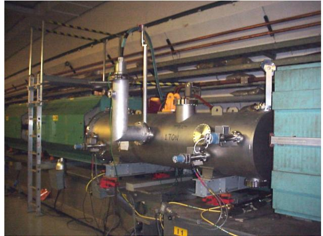
Figure 2: The New AGS Electro Static Septum
