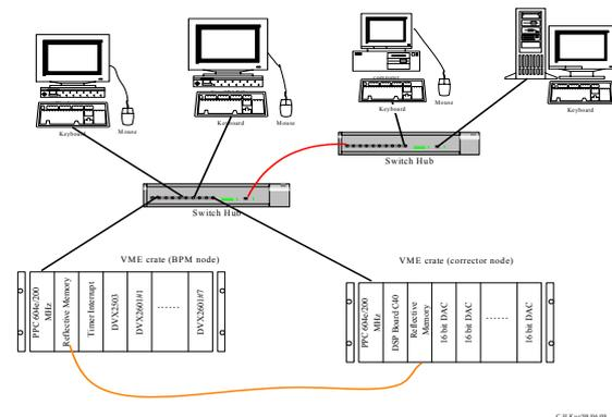
Figure 1: Original hardware environment of the orbit feedback system.
