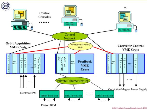
Figure 3: Hardware structure of the orbit feedback system.
