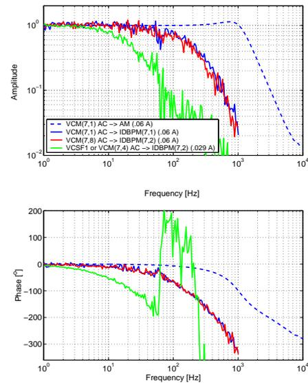
Figure 3: Transfer function of an ALS corrector magnet power supply and combined transfer function of power supply, magnet, vacuum chamber and beam.
