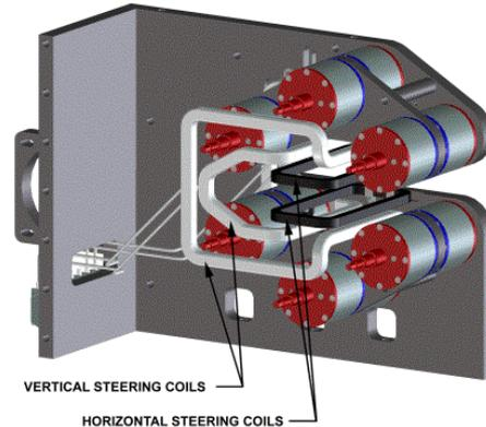
Figure 1: New permanent magnet/air coil chicane magnets.
