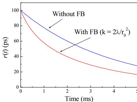
Figure 3: Calculated damping effect due to the feedback. Assumed  $r_0 = 100$  ps,  $\lambda = 255$  s<sup>-1</sup>, and  $\Delta\phi = \pi/2$ .
