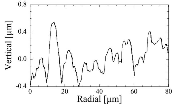
Fig 2: Cathode surface cross-section profilometry plot.
