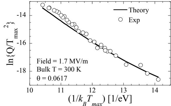
Fig. 6: Demonstration that current follows *field & photo-enhanced thermal emission model* (Eq. (3)). Max temperature evaluated via Eq. (1) for center of laser pulse.
