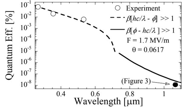
Fig. 1: Measured QE at various  $\lambda$  for Scandate dispenser cathode. Lines refer to Eq. 4. Black dot = same in Fig. 3.
