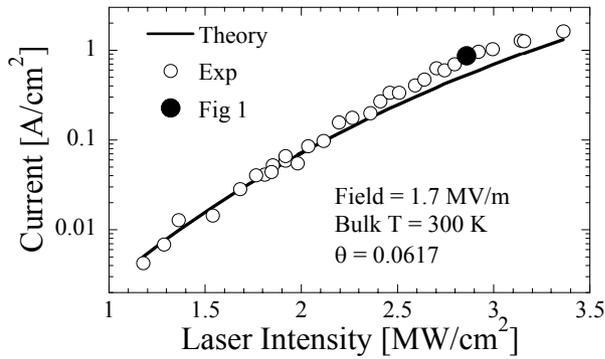
Fig. 3: Current Density vs. laser intensity.
