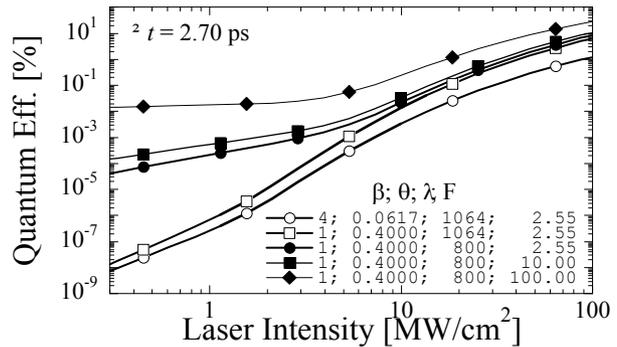
Fig. 7: Extrapolation for other  $\theta$ ,  $\lambda$ [nm] and  $F$ [MV/m] for Scandate cathode.  $\beta=1$  means no field enhancement
