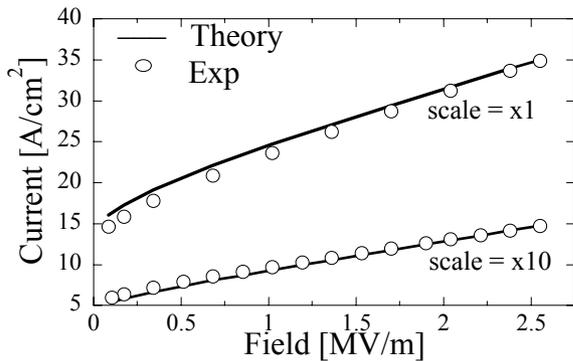
Fig. 5: Same as Figure 3, but for variation in field (top) 5.3 MW/cm<sup>2</sup>, 713 K; (bottom) 2.9 MW/cm<sup>2</sup>, 633K
