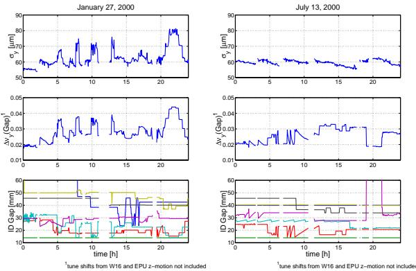
Figure 4: Vertical beamsize changes versus insertion device gap motion before (left) and after (right) tunefeedforward was implemented.
