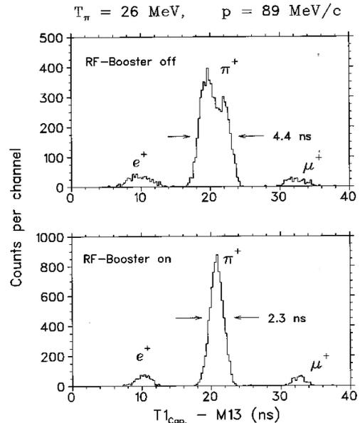
Figure 5: The  $e^+ \pi^+ \mu^+$  time distribution at the CHAOS detector with and without rf booster.
