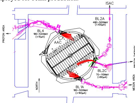
Figure 3: Layout of the cyclotron vault and of four systems for simultaneous extraction.
