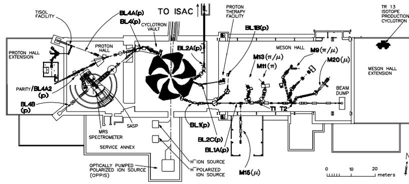
Figure 1: Layout of the cyclotron facility.
