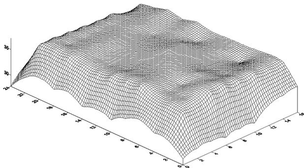
Fig. 5. Measured magnetic flux density profile
