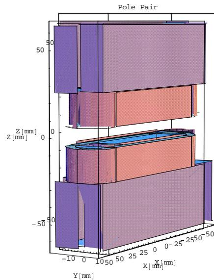
Figure 2: Schematic layout of a pole pair in the MAX-Wiggler, showing the coils, the iron central cores and the return yokes.
