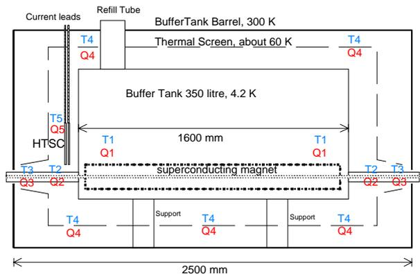
Figure 5: Schematic layout of the cryogenic system of the MAX-Wiggler cryostat.
