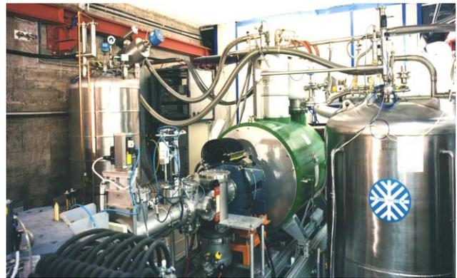
Figure 1: A recent photo of the SERSE source and of the first section of its beamline.
