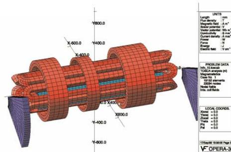
Figure 5: A sketch of the GyroSERSE magnets (courtesy of ACCEL Instr. GmbH).
