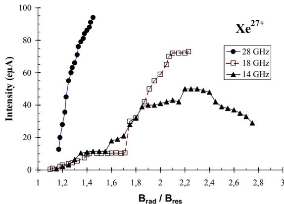
Figure 2:  $Xe^{27+}$  currents obtained by operating SERSE at different frequencies versus increasing radial field.
