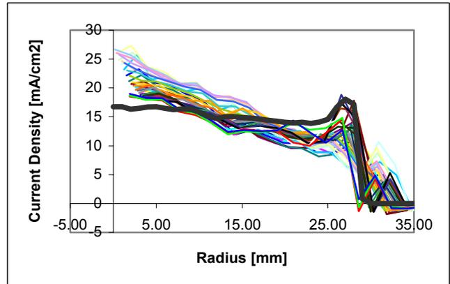
Figure 4. Measured beam profiles for an 80-kV equivalent (extractor) beam at an axial distance of 2.54 cm, and EGUN predicted profile (thick black curve).
