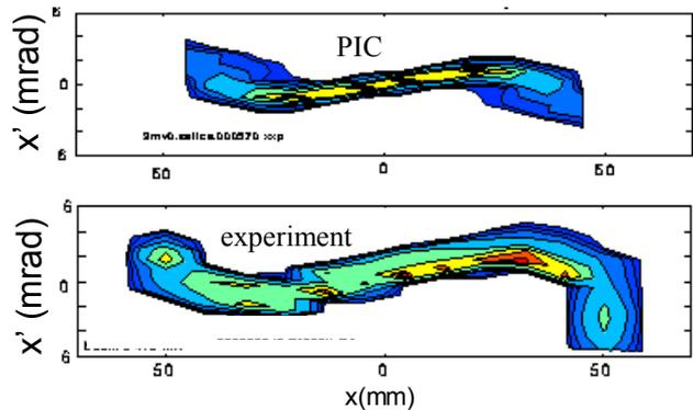
Figure 7. Transverse phase space calculated (PIC) and measured at the exit of the ESQ injector for 80 kV (equivalent) extractor voltage.
