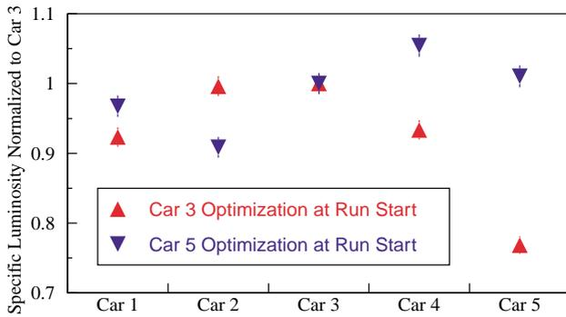
Figure 3: The car by car performance (averaged over all trains) when the electron-positron differential vertical displacement was adjusted at the start of the run to maximize the BBI luminosity signal for car 3 and car 5.
