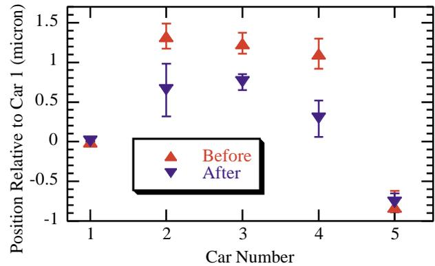
Figure 4: Positron - electron differential positions averaged over all trains relative to the average bunch 1 differential position before and after adjusting the vertical positioning of all bunches using the feedback system's kicker.
