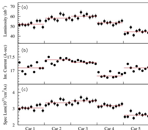
Figure 2: The (a) integrated luminosity, (b) integrated current, and (c) run-averaged specific luminosity of an HEP run where there were 9 trains of 5 bunches. The points represent the performance for individual cars while the lines indicate the average over all trains for each car.
