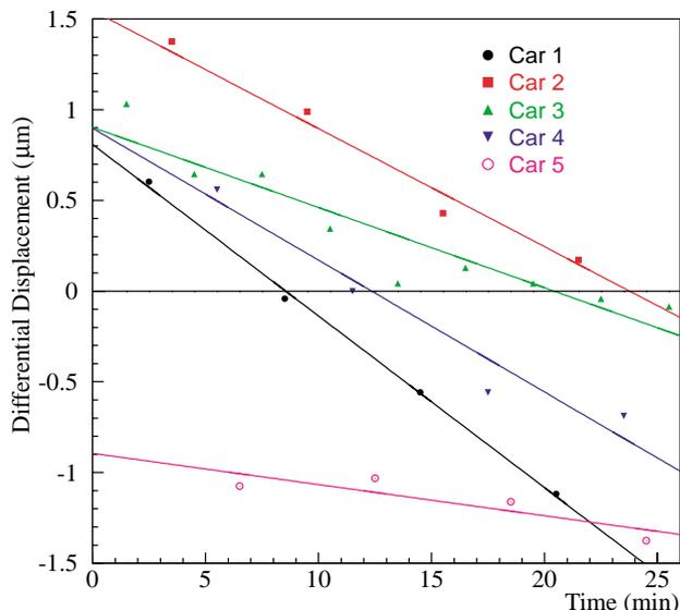
Figure 1: The vertical differential displacement for head-on collisions as a function of time as determined by maximizing the BBI Luminosity Monitor signal. Car #1 refers to the 9 leading bunches in the 9 trains, etc. The lines are linear fits to the data. The zero of the vertical axis is arbitrary.
