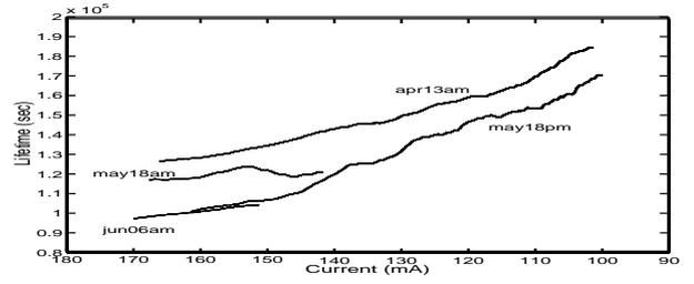
Figure 3: Beam lifetime for the normal operation period, *apr13am* and abnormal beam lifetime reduction due to the various RF noise-sidebands
