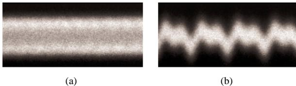
Figure 5: Streak camera images (a) when there is no RF noise-sideband. (b) when 10 hour beam lifetime reduction is generated due to RF noise-sidebands. Maximum horizontal time scale is 1 ms, and vertical time scale which means the bunch length is same for two cases.
