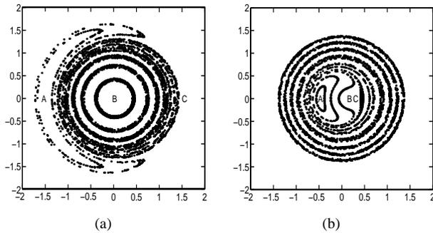
Figure 4: Phase space tracking of the RF phase modulation for (a) *may18am*, (b) *may18pm*. Here the horizontal and vertical axes mean  $\sqrt{2\tilde{J}} \cos(\tilde{\psi} - \nu_m \theta)$  and  $\sqrt{2\tilde{J}} \sin(\tilde{\psi} - \nu_m \theta)$ , respectively.
