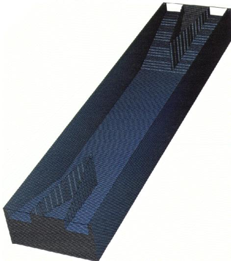
Figure 7: The wedge model generated by the MAFIA used for studying the trapped modes. Dimensions for the
