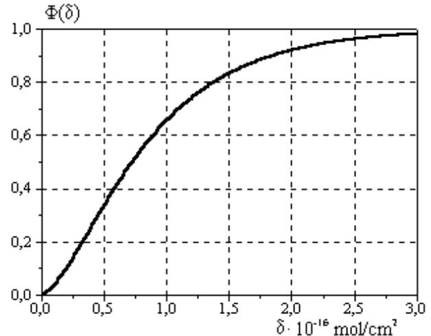
Figure 2: Dependence of the conversion coefficient on the target thickness.
