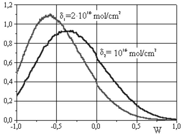
Figure 5: Distribution of the proton energy spread for the different target thicknesses, in the case of the Gaussian distribution of the gas density.
