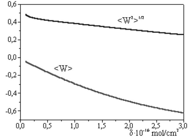
Figure 4: Dependence of the mean change of proton energy  $\langle W \rangle$  and the mean-square energy spread  $\langle W^2 \rangle$  on the target thickness.
