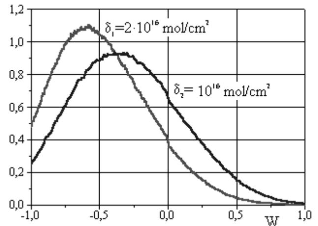
Figure 5: Distribution of the proton energy spread for the different target thicknesses, in the case of the Gaussian distribution of the gas density.
