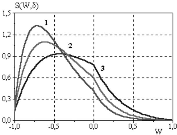
Figure 3: Distribution of the proton energy spread for the different target thicknesses. Curves 1, 2, 3 show results for  $\delta = 2 \cdot 10^{16} \text{ mol/cm}^2$ ,  $1.5 \cdot 10^{16} \text{ mol/cm}^2$ ,  $1 \cdot 10^{16} \text{ mol/cm}^2$ , respectively.
