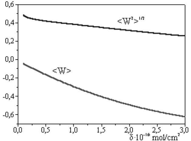
Figure 4: Dependence of the mean change of proton energy  $\langle W \rangle$  and the mean-square energy spread  $\langle W^2 \rangle$  on the target thickness.
