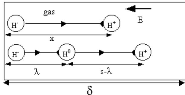
Figure 1: The schematic plot of the exchange ion  $H^- \rightarrow H^+$  process on the gas target.
