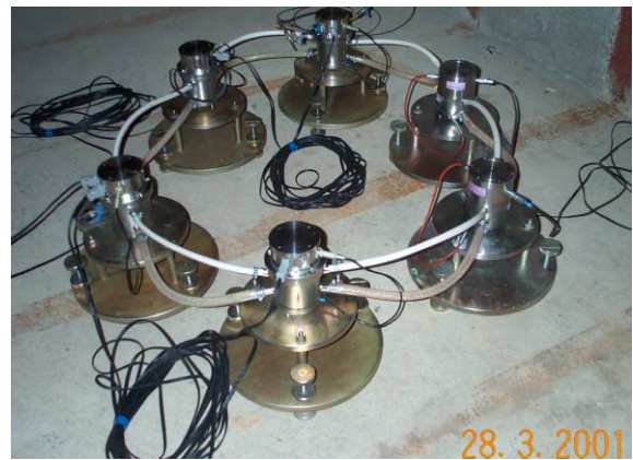
Figure 3: Four SAS and two Fogale probes in the dual tube configuration placed close together to measure system noise.
