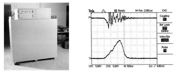
Figure. 3. Left: Opening switch delivered to CPI. Right: Waveforms of a deliberate short. Upper trace, voltage, 50kV/division; lower trace, current, 250 A/division.
