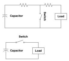
Figure 1. Circuit diagrams for crowbar (upper) and opening switch (lower).
