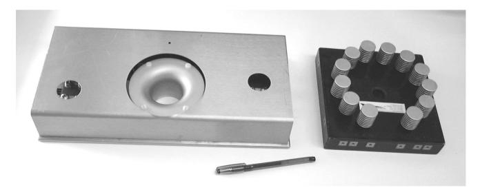
Figure 4. Switch modules. Left: 3kV high-current (65A DC, 750A pulsed). Right: 6kV low-cost (25A DC, 250A pulsed).
