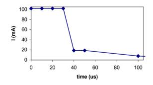
Figure 2. Beam current vs. RF interruption. An interruption of up to 30 µs can be sustained without beam loss.
