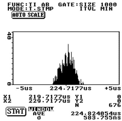
Figure 6. Chopper-tracking histogram of the controller with the chopper simulator. Ref. at level 2.
