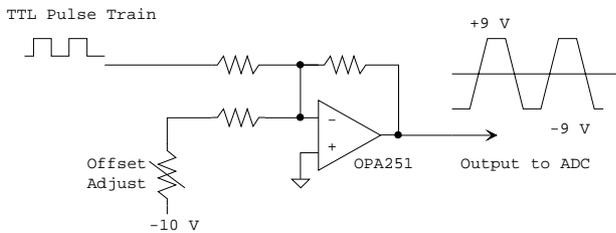
Figure 2. Simplified schematic of a slew-rate limiting circuit.
