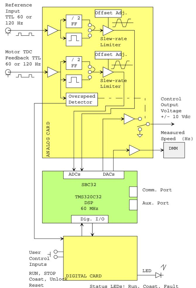
Figure 1. Simplified block diagram of the neutron chopper speed and phase controller.
