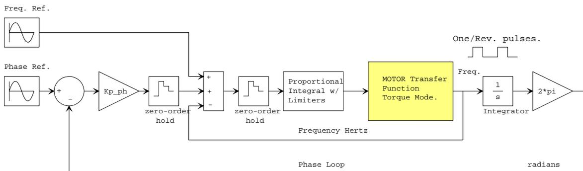
Figure 3. Simulink control-system model of the speed and phase controller.
