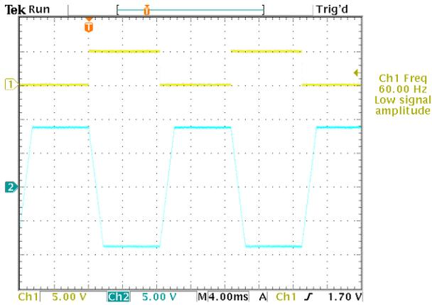
Figure 4. Picture of a TTL input and slew-rate limited output signal. Top: Input TTL signal. Bottom: Slew-rate limited signal ranging from about -9 to +9 volts.
