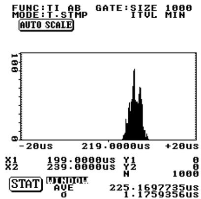
Figure 7. Chopper-tracking histogram of the controller with the chopper simulator. Ref. at level 5.
