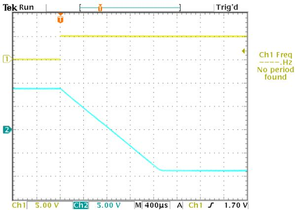
Figure 5. Expanded scale of figure 4. Top: Input TTL signal 0 to ~5 V. Bottom: Slew-rate limited signal showing fall time of about 1.7 ms.
