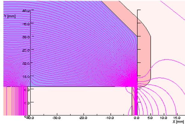
Figure 3: Magnetic flux distribution for an eddy-current Cu-Fe septum magnet at the end of the current pulse (0.4 ms) when the gap field is zero.
