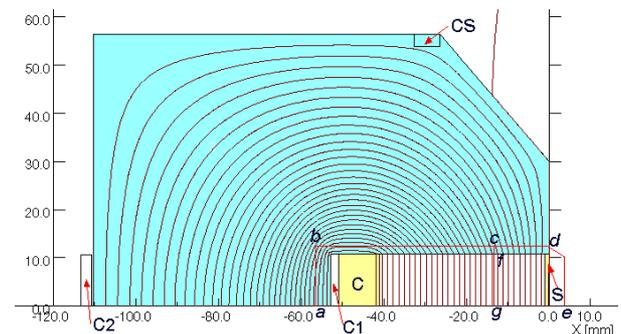
Figure 1: Cross section of the upper half of a direct-drive septum magnet with its magnetic flux distribution. C and S: main coil and septum conductor. C1 and C2: correction coils. CS: correction coil for S. Lines abcd and de denote the line integral paths ad and de in Eq. (1), and gf is the half-gap of the magnet.
