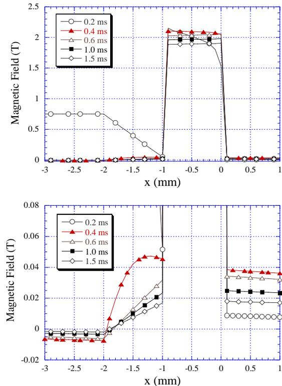
Figure 4: Magnetic fields near the 2-mm Cu-Fe septum ( $-2.0 \leq x \leq 0$ ) of an eddy-current septum magnet were calculated during and after the current pulse. The fields in the steel septum are over 2 T (*top*), and the leakage fields are shown in expanded scale for the vertical axis (*bottom*).
