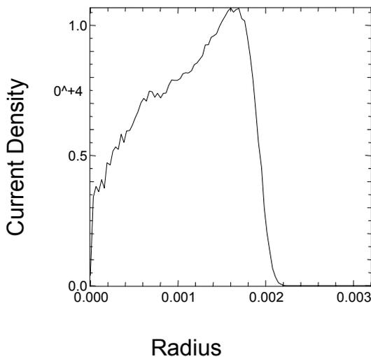
Fig 3. Radial variation in current density when the injected current is increased 50% to 207 mA.
