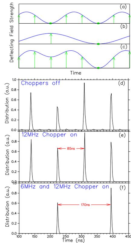
Figure 6: (a) Output time structure from the RFQ is shown in (d). The field produced by the 11.8 MHz chopper plate (a) produces a 85 ns time structure shown in (e). The field produced by the 5.9 MHz plate in (b) is combined with the 11.8 MHz deflection to produce the combined deflection shown in (c) and generates the time structure given in (f).
