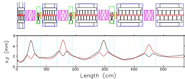
Figure 7: Schematic of the ISAC DTL showing five IH accelerating tanks, four quadrupole triplets and three triple gap bunchers. The transverse beam envelopes are also plotted.
