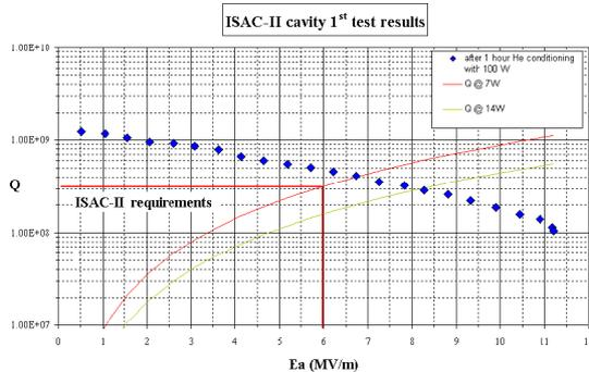
Figure 12: First rf test results for the prototype 106.1 MHz medium- $\beta$  cavity for ISAC-II.
