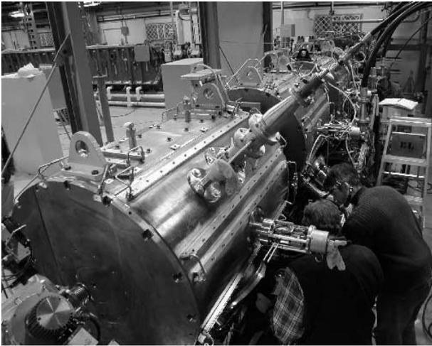
Figure 8: The ISAC 106 MHz DTL.
