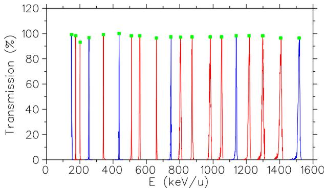
Figure 9: We plot the measured transmission for the various beams that have been accelerated through the DTL during commissioning studies with  $^4\text{He}$ .
