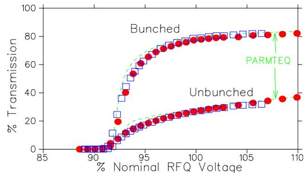
Figure 5: RFQ beam test results showing capture efficiency for beams of  $^{14}\text{N}$  (squares) and  $^{14}\text{N}_2$  as a function of relative vane voltage. The beam capture for both bunched and unbunched initial beams are recorded (squares) and are compared with PARMTEQ calculations (dashed lines).
