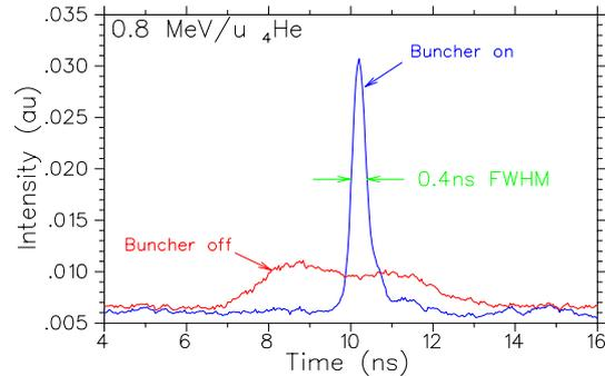
Figure 10: Beam time distributions measured on a fast Faraday cup near the DRAGON target for high  $\beta$  buncher off and on.
