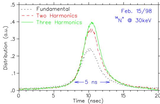
Figure 3: Time distribution of beam measured on a fast Faraday cup upstream of the RFQ for one, two and three harmonics on the LEBT prebuncher.
