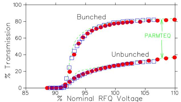
Figure 5: RFQ beam test results showing capture efficiency for beams of  $^{14}\text{N}$  (squares) and  $^{14}\text{N}_2$  as a function of relative vane voltage. The beam capture for both bunched and unbunched initial beams are recorded (squares) and are compared with PARMTEQ calculations (dashed lines).
