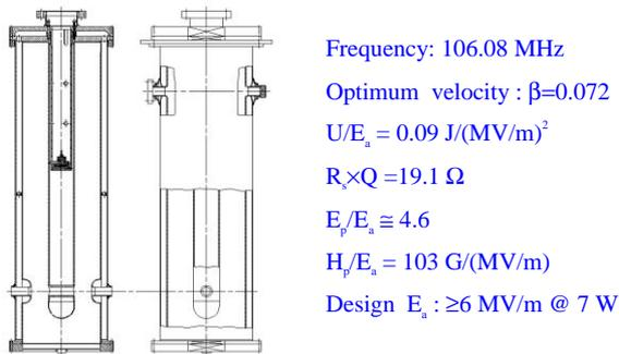
Figure 11: The prototype 106.1 MHz medium- $\beta$  cavity for the ISAC-II project at TRIUMF.
