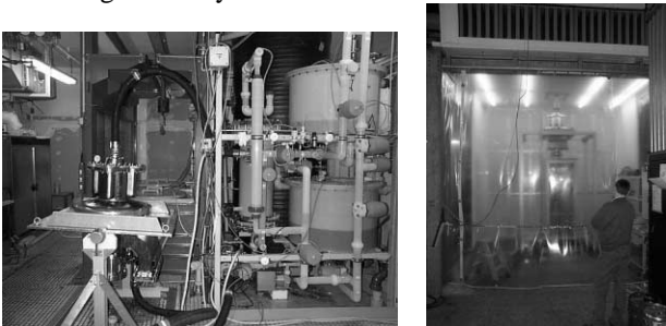
Figure 2: Preparation of the first cavity for a vertical test. Left: closed loop BCP, right: high pressure rinsing.
