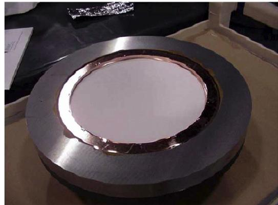
Figure 6. Fixtured window assembly ready for braze.
