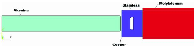
Figure 5. Material configuration for the window braze.
