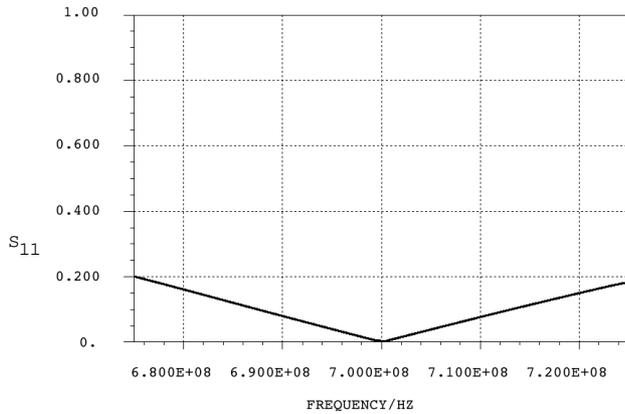
Figure 3. Calculated  $S_{11}$  of LEDA waveguide window.
