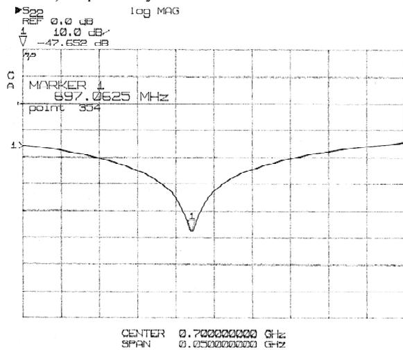
Figure 8. Window final frequency measurement in spool.
