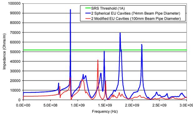
Figure 3. Cavity Transverse HOM Spectrum.
