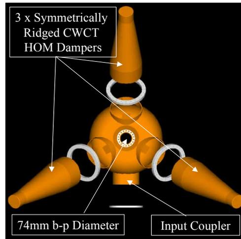
Figure 1. Spherical EU Cavity Design Assembly.
