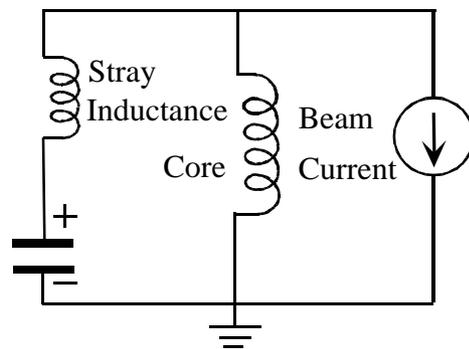
Figure 2: Equivalent circuit of induction module with beam loading
