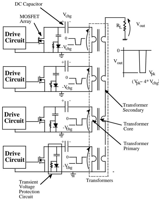
Fig. 3: Simplified circuit schematic for the voltage-adder concept.
