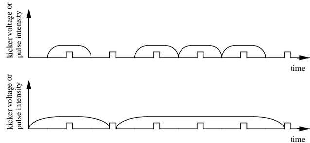
Figure 2: Extraction of adjacent bunches with constant-width (upper graph) and stretched (lower graph) pulses.
