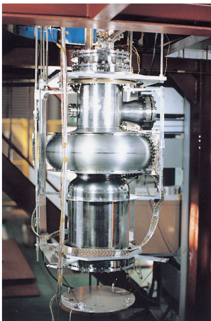
The superconducting cavity prepared for vertical testing
