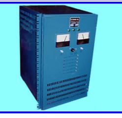
CERN, GENEVA, SWITZERLAND 9200 SERIES POWER CONVERTERS ONE QUADRANT WITH REGENERATION TOPOLOGY: Soft Switching IGBT INPUT: 400/3/50 VAC OUTPUT: 550 VDC @ 450A, 250kW STABILITY: +/- 50ppm Low EMI, Low Ripple, Fast Response OPTIONAL: Four Quadrant Operation : Power Regeneration
