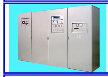
SCANDITRONICS MEDICAL, SWEDEN 9200 SERIES POWER CONVERTERS FOUR QUADRANT, 12 PULSE RECTIFIER TECHNOLOGY: Intelli-mod IGBT INPUT: 400/3/50 VAC OUTPUT: +/-200 VDC @ +/-15A, 3kW STABILITY: <+/-1000ppm FEATURES: Low EMI Emissions : Low Input Harmonics
