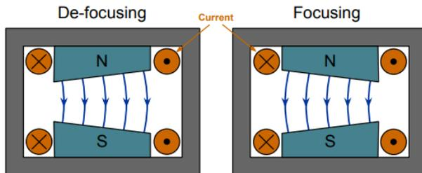
Fig. 1: Schematic of the combined function magnets.
