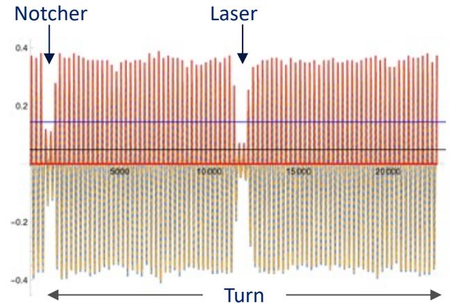
**Opposite-notch** structure with laser notcher misaligned from the notch kicker by 42 buckets.
