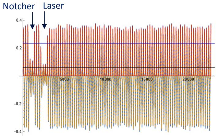
**Double-notch** structure with laser notcher misaligned from the notch kicker by 6 buckets.
