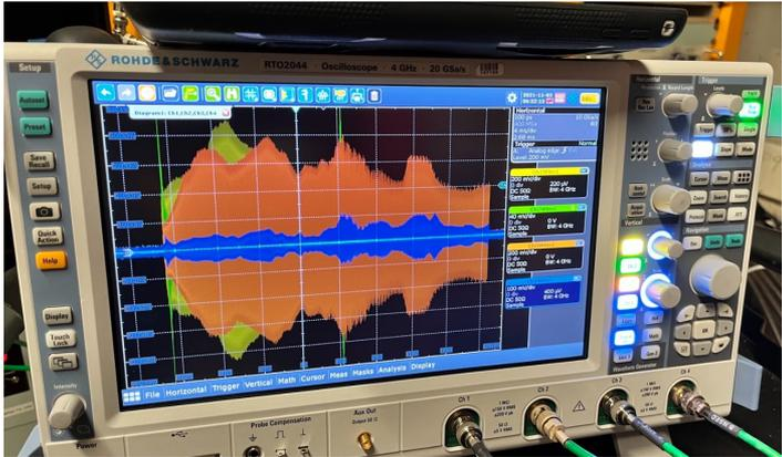
Fig. 6: Scope signal includes horizontal sum and difference, vertical sum and difference.
