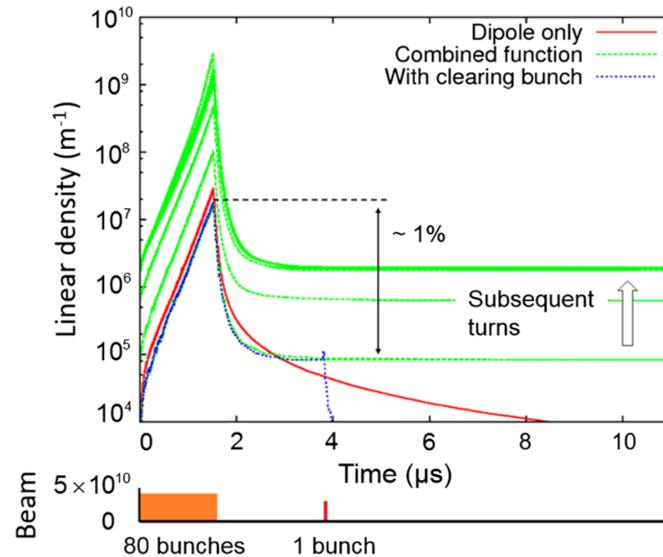
In a combined function magnet, the electron cloud accumulates over many revolutions, reaching a much higher density, than in a pure dipole. A clearing bunch destroys the trapped cloud, preventing the accumulation.
