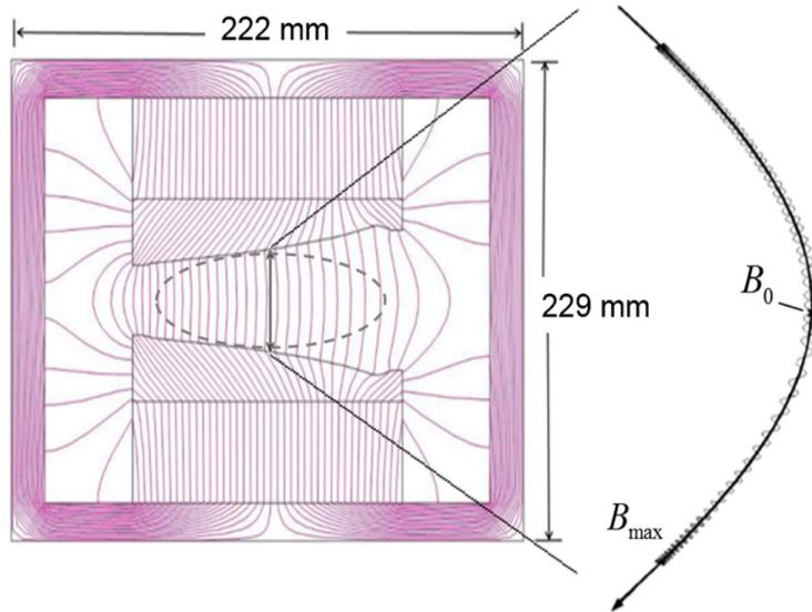
Fig. 3: Field lines inside a combined function magnet.
