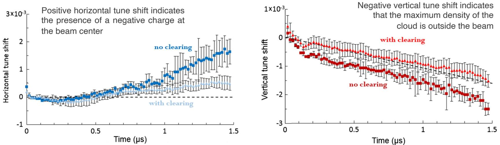
Fig. 7: Betatron tune shift within the 80-bunch train with respect to the first bunch, measured over 600 revolutions with a stripline detector in the Recycler.
