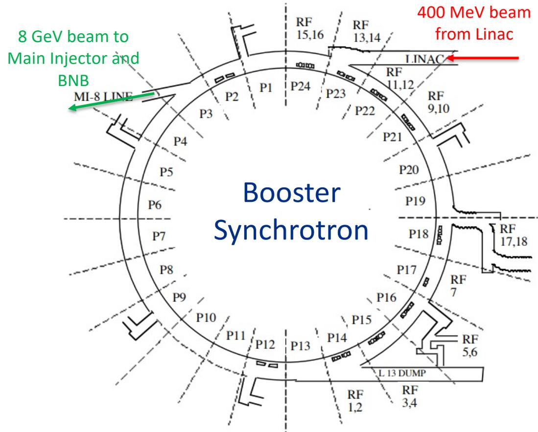
Fig. 2: Schematic of the Fermilab Booster synchrotron.
