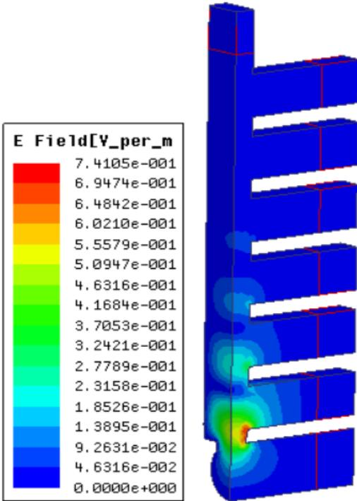
$E$ -field structure of the operating eigenmode.
