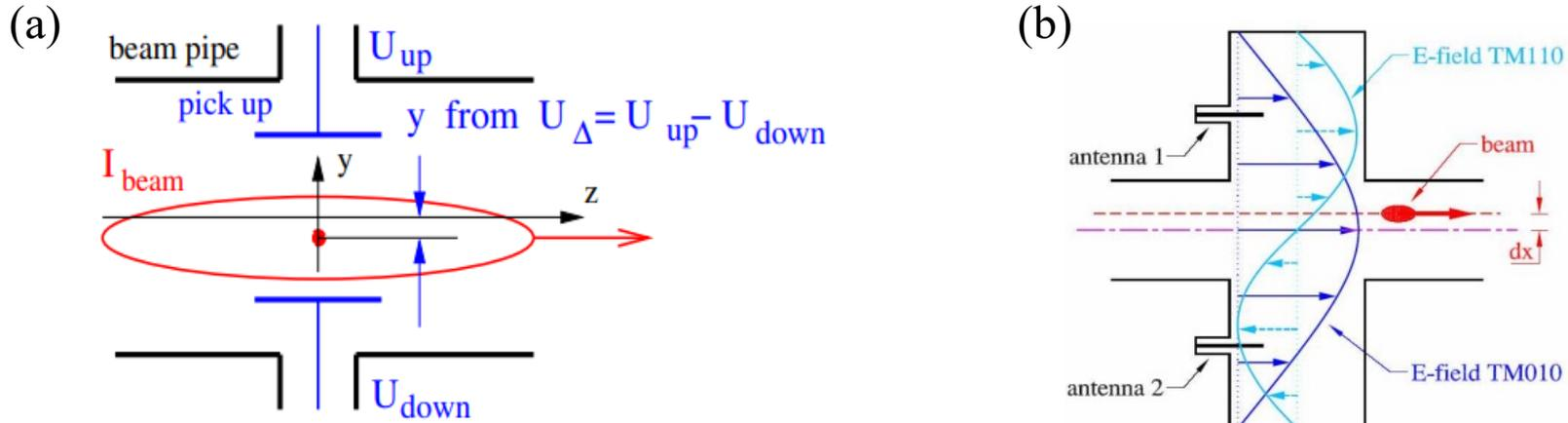
Classical button BPM based on proximity effect (a) and pillbox cavity BPM (b). [P. Forck, et al. CERN Accelerator School 2009.]
