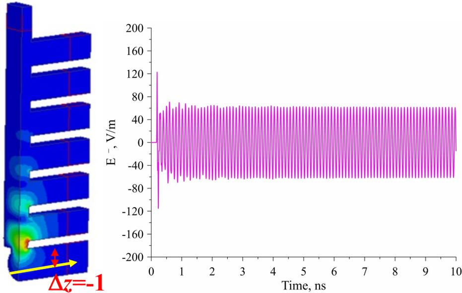
$E_x$ -field component at the PBG resonator when excited by a bunch shifted by  $\Delta z = -1$  mm from the  $x$  axis.
