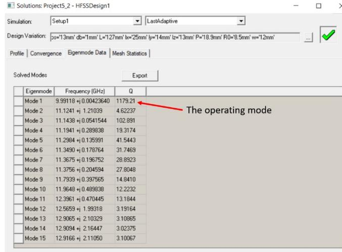
Eigenmodes of the resonator.
