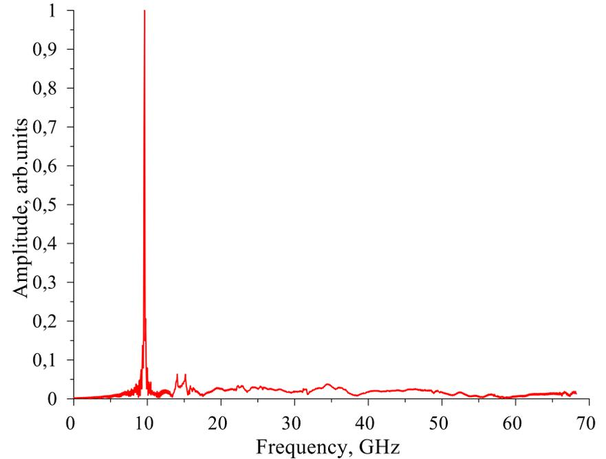
Fourier spectrum for the field excited in the resonator.
