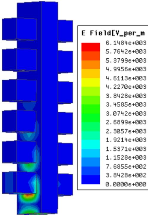
E-field structure of Bragg reflector at 10 GHz.
