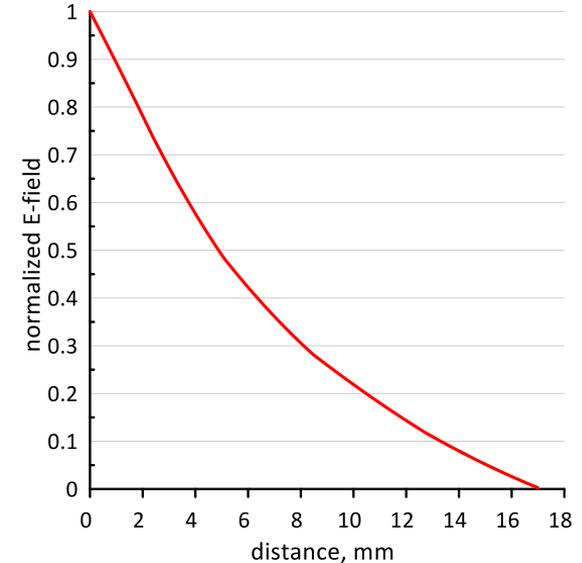
$E_x$ -field near the coupling hole across the beam line.
