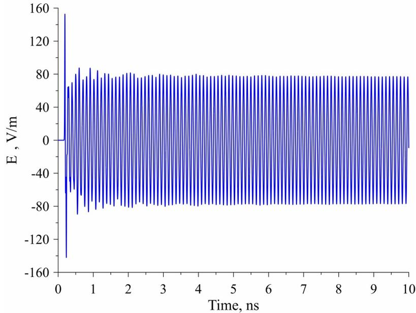
$E_x$ -field component at the resonator when excited by a bunch moving along the  $x$  axis.
