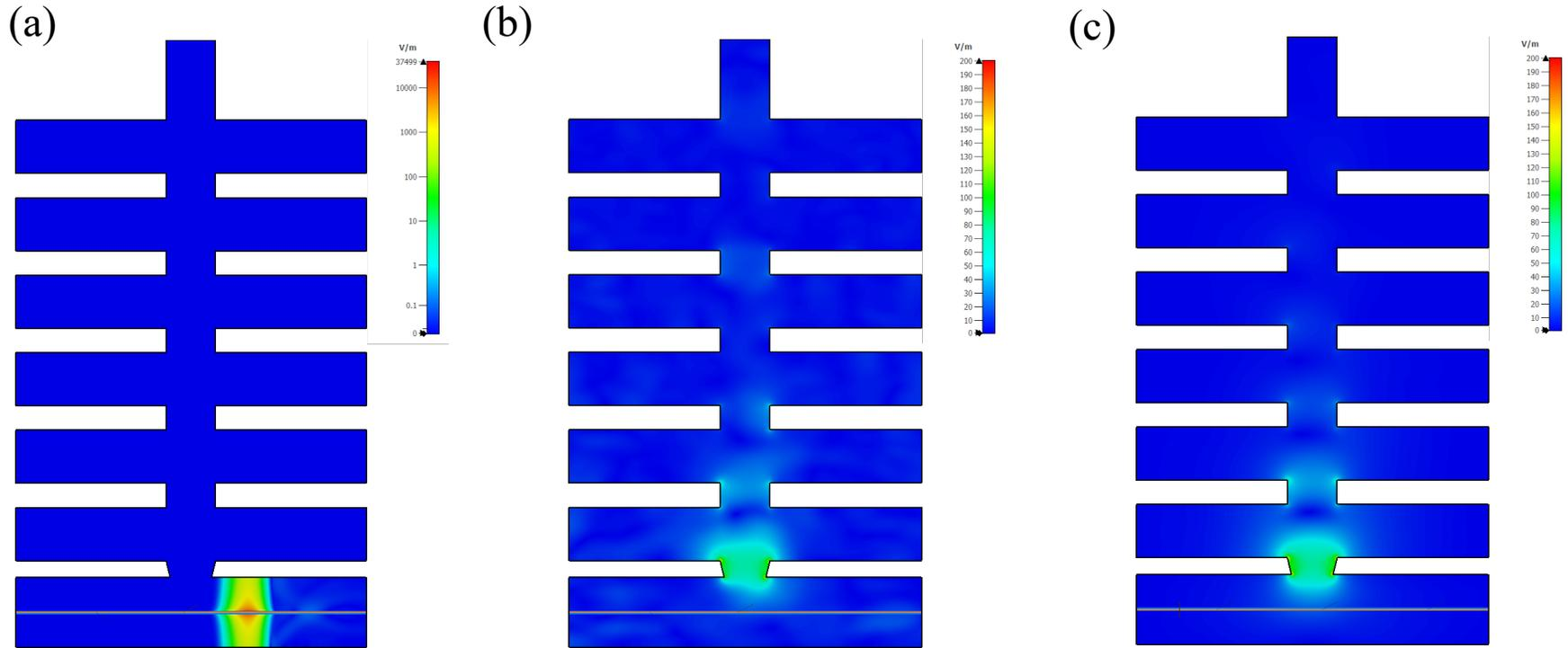
Instantaneous field distribution in the PBG resonator: a – the bunch approaches to the resonator, b – 1 ns after the bunch leaves the coupling area, c – 10 ns after the bunch has passed. The bunch length was set as 10 ps, the charge was 1-pC.
