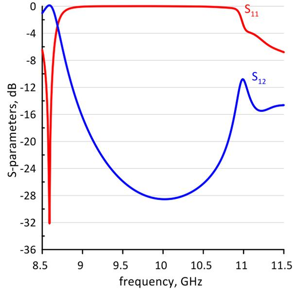
S-parameters of Bragg reflector vs. frequency.
