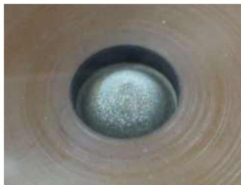
Electroplated Ra (1 mCi) on conical Au surface **
