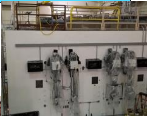
Newly refurbished hot cells for alpha-processing
