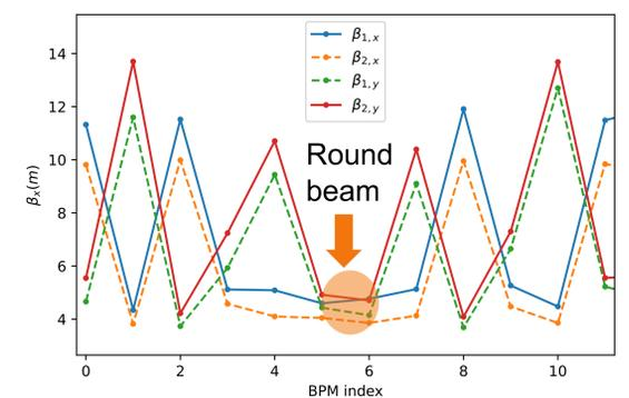
Measured coupled Twiss for one supercell
