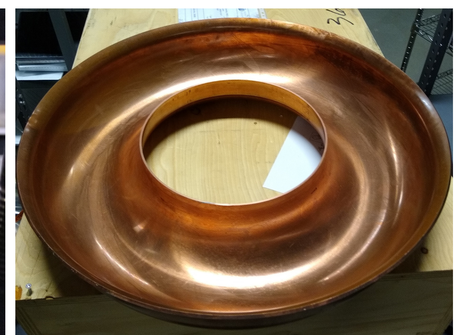
“short plate” hydroforming test
