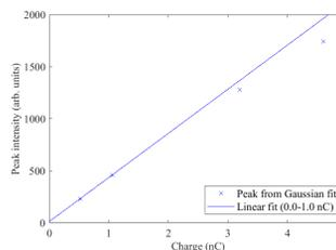
Figure 4: Intensity as a function of peak charge areal density.
