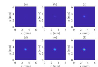
Figure 6: Fitted electron beam sizes as a function of electron beam charge.
