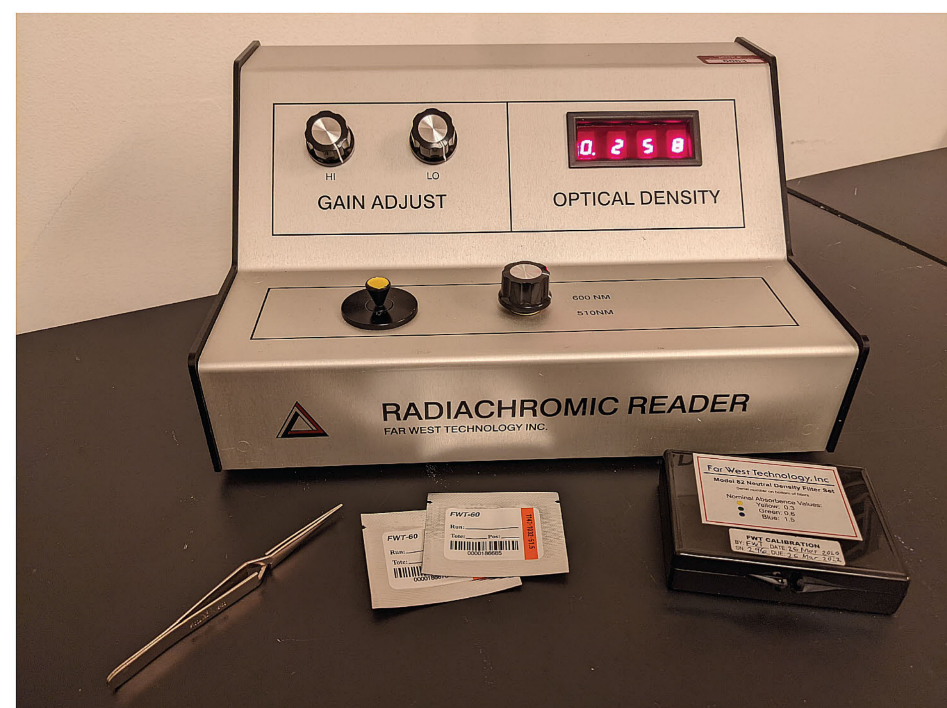
FWT-92D Film Reader and FWT-60 film pouches.
