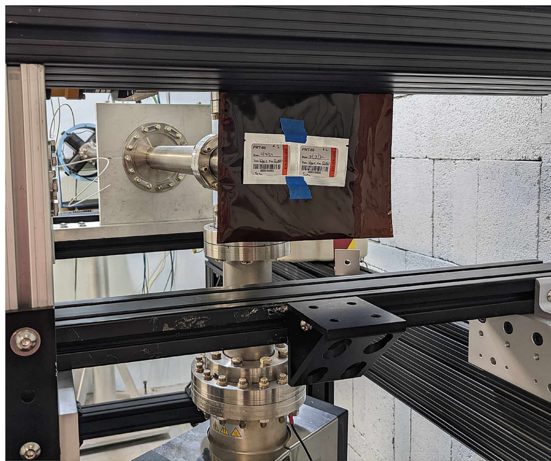
Film sheet in UV protective bag positioned for beam imaging.
