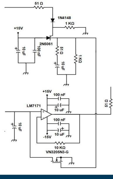
The 1N4148 allows only the positive cycle of the differentiator to cross and trigger the gate of the 2N5061 SCR.
