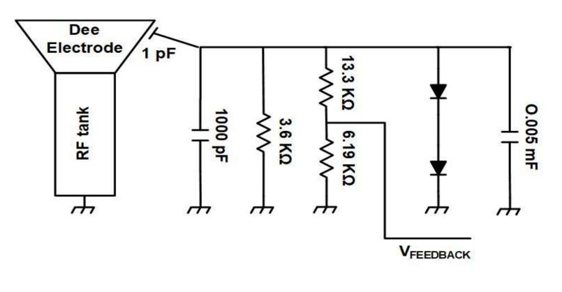
The probe consists of an isolated flush plate that faces the Dee electrode and has a 1 pF capacitance to the Dee electrode. A 1000 pF capacitor is connected to the plate to sample the RF, working as a 1/1000 divider. A resistor divider of 13.3 K $\Omega$  and 6.19 K $\Omega$ decreases the amplitude further, producing <u>a feedback voltage, V<sub>FEEDBACK</sub>, that is sent to</u> the Dee voltage regulator.
