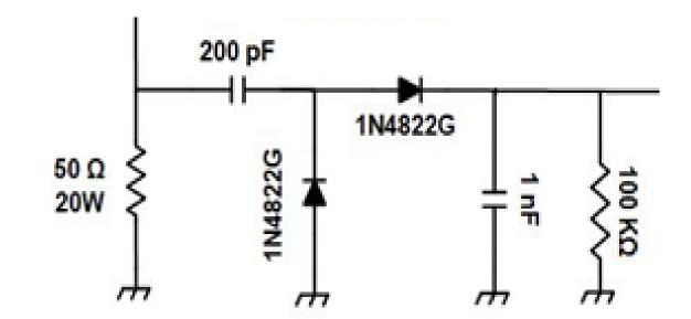
The peak-to-peak detector is a combination of two cascaded parts:
