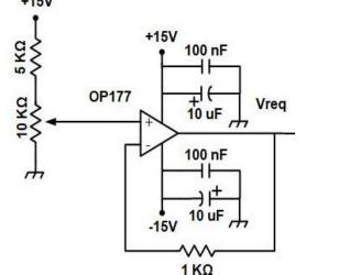
A 10 K $\Omega$  potentiometer gives the <u>reference voltage</u> that is buffered by the OP177 Ultraprecision Operational Amplifier and compared to the voltage from the peak-topeak detector.
