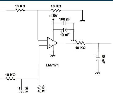
The reference voltage is applied to the positive input of the LM7171. The peak-to-peak voltage is applied to the negative input of the LM7171. If the signal from the peak detector is above the requested voltage, the output voltage will decrease and the GC2001C attenuation will increase (or vice-versa), regulating the amplitude of the RF.
