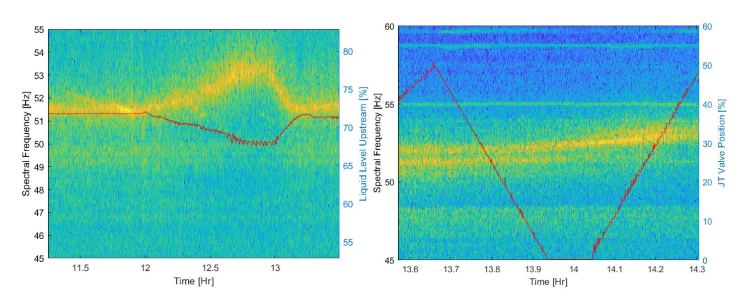
mode in cavity 1 CM21. The liquid level is correlated with the 51.5 Hz mode
