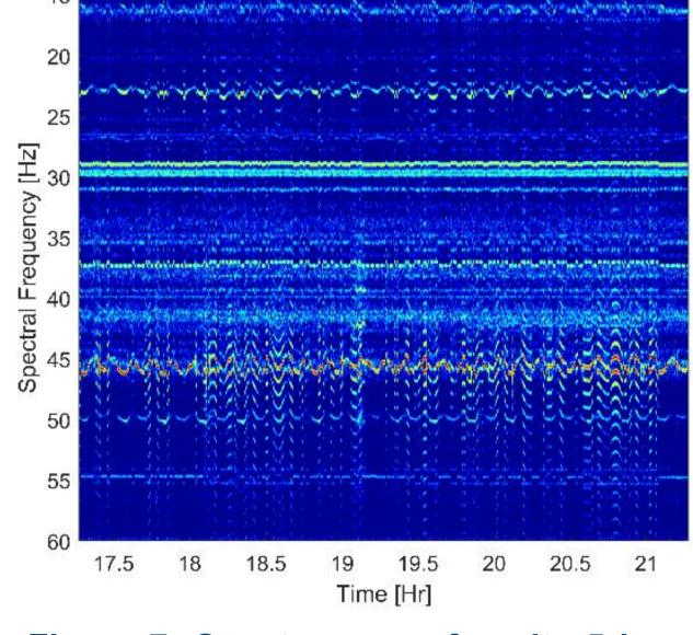
Figure 7: Spectrogram of cavity 5 in CM15 showing the harmonics with fundamental frequency of 23 Hz and higher order frequency of 46 Hz. .
