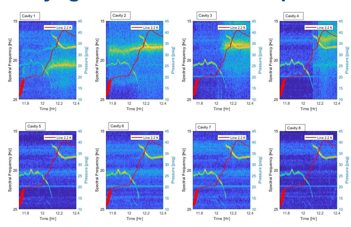
Figure 5: Spectrogram of the cavities in vCM showing the transition of 20 Hz vibration to 18 Hz by changing the supply pressure of the 2.3
