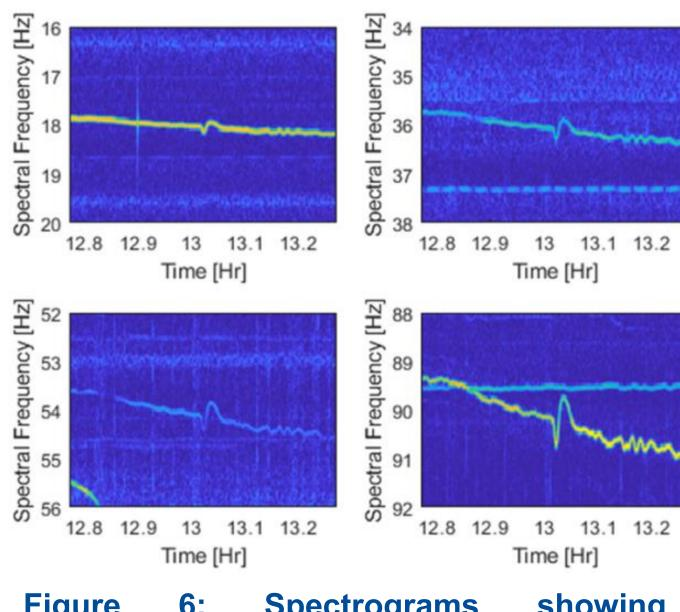
**Spectrograms** showing harmonics observed in cavity 7 in CM 15, the fundamental mode occurs at 18 Hz.
