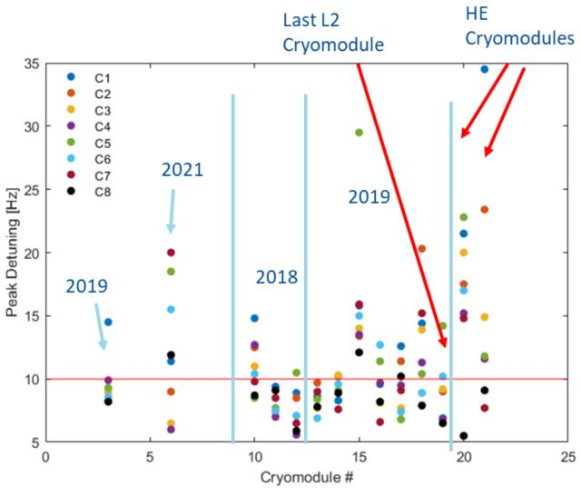
Figure 3: Cavity peak detuning of all 8 cavities from cavities tested from 2018 until 2022. These include cavities from LCLS-II and HE. The cavity peak detuning specification is 10 Hz.
