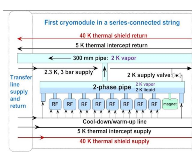
Figure 2: Cryogenic flow schematic of a 1.3 GHz LCLS-II cryomodule.
