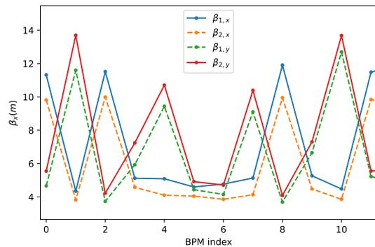
Figure 5: Measured Ripken Twiss parameters for one supercell (cell 30 and 1). Here the round beam was obtained at the short straight section between BPM 5 and 6.
