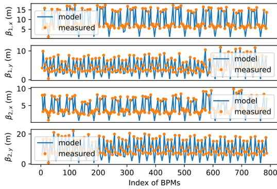
Figure 3: Comparison of the Ripken Twiss functions between the lattice model and the extraction from simulated TbT data.
