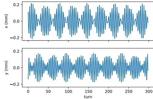
Figure 2: Simulated TbT data at one BPM.
