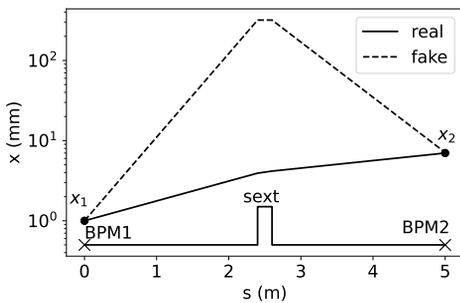
Figure 1: Reconstruction of trajectory with a sextupole located between two BPMs. Given only BPM readings, there may be more than one possible trajectory, but the paraxial trajectory is real.
