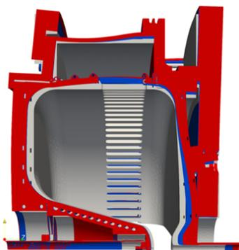
Figure 7: The deformed Gun-2 cavities with a 2.3 (red) and a 4.0 (blue) gpm anode flow rates for a cathode gradient of 20 MV/m and undeformed Gun-2 cavity (grey). The geometry deformations are scaled 100 times large for visualizing.
