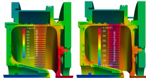
Figure 6: The temperature profiles with a 2.3 (left) and 4.0 (right) gpm anode flow rates in Gun-2 solid model for a cathode gradient of 20 MV/m.
