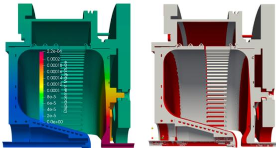
Figure 5: Gun-2 displacement amplitude (left) and geometries (right) without (grey) and with (red) atmospheric pressure. The geometry deformation is scaled 100 times large for visualizing.
