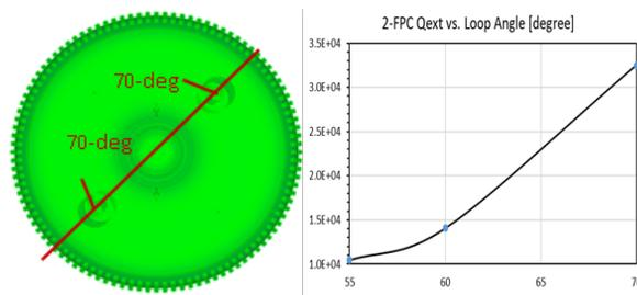
Figure 1: The Gun-2 3D geometry showing the couplers and their loop orientations at the critical coupling (left) and  $Q_{ext}$  versus the loop angle in degrees (right).
