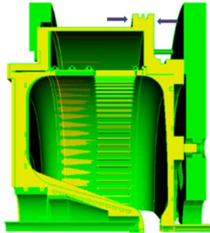
Figure 4: An overlay of the Gun-1 (yellow) and Gun-2 (green) solid models.
