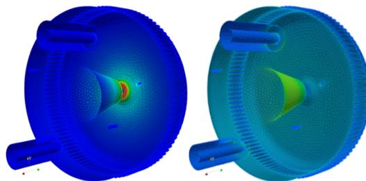
Figure 2: The complex electric (left) and magnetic (right) fields in the Gun-2 3D geometry when  $Q_{ext} = Q_0$ .
