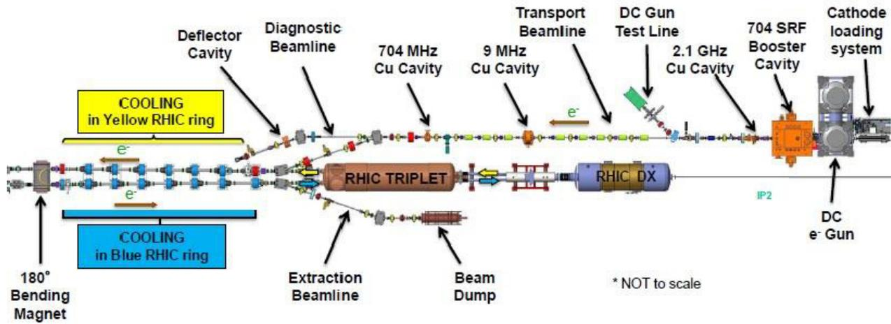
Figure 2: Layout of the LEReC accelerator.
