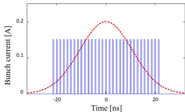
Figure 1: The LEReC beam structure. Thirty electron bunches (blue) spaced by 1.4 ns placed on a single ion bunch (red), with ion bunch repetition frequency of 9 MHz.
