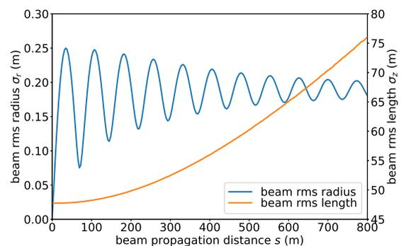
Figure 1: Evolution of the rms radius and the rms beam length of the simulated pulsed electron beam generated by the Beam-PIE experiment as it propagates parallel to the background magnetic field.
