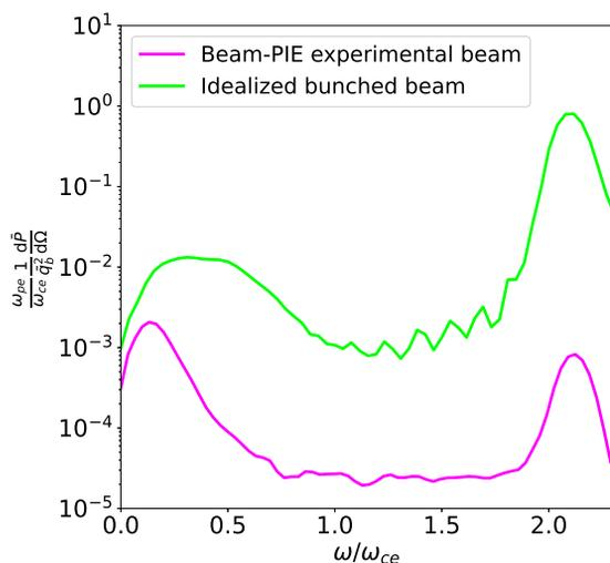
Figure 4: Spectra of the plasma wave radiation by a single electron bunch in the case of the Beam-PIE electron beam (magenta) and of the idealized bunched beam (lime), normalized by the beam charge, plotted versus the normalized frequency  $\Omega = \omega/\omega_{ce}$ .
