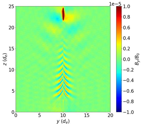
Figure 3: The field pattern of the plasma wave generated by the idealized bunched electron beam at a propagation distance of 362.1 m, represented by the distribution of  $B_y/B_0$ . The beam shown spans from  $z = 21.3 d_e$  to  $z = 25.0 d_e$ .
