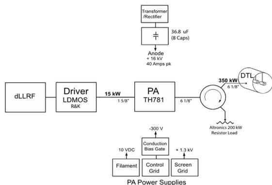
Figure 2: Diagram of New RF Amplifier System.
