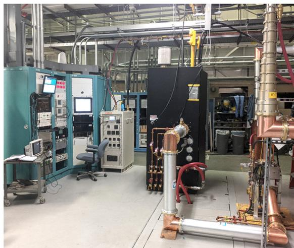
Figure 3: From left to right: LLRF, cRIO controller, SSA, PA (black unit), Circulator (end view) and Load (vertical).
