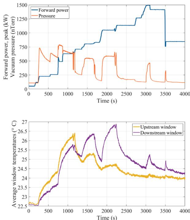
Figure 3: Peak forward power into the WTS and the vacuum pressure vs time (top), and the upstream and downstream window temperatures averaged over all IR sensors (bottom).
