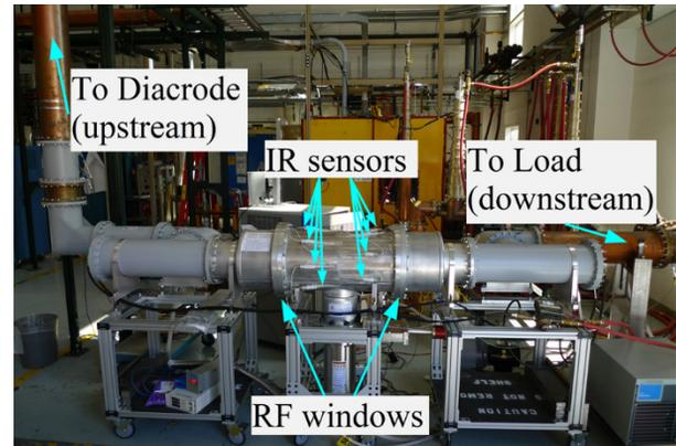
Figure 1: The window test stand in place for testing.
