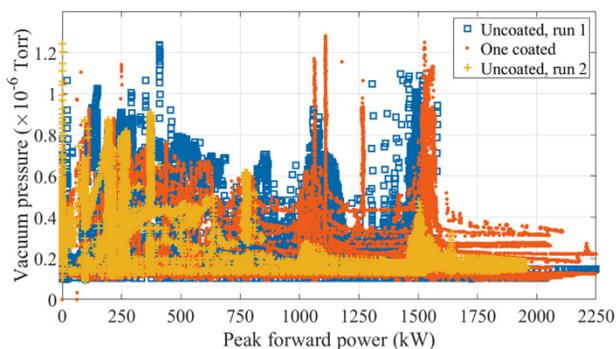
Figure 2: Vacuum pressure vs the peak forward power into the WTS for all three window configurations.
