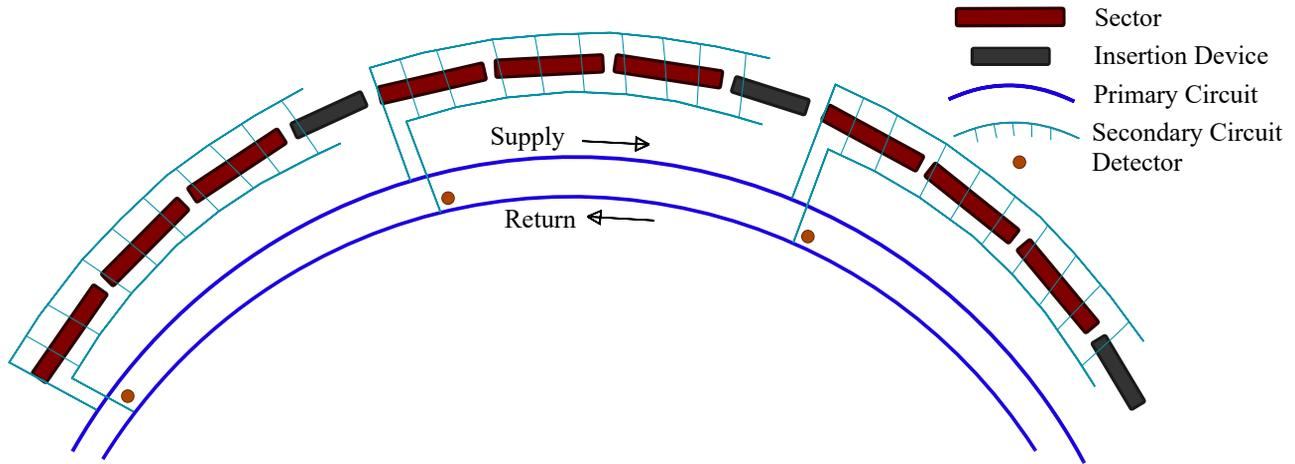
Figure 1: Schematic illustration of primary and secondary water systems. With approximately one secondary system per machine sector, detectors can be placed at each connection to the primary circuit to provide segmented coverage of the entire ring. Short flexible hoses supply and return water from individual accelerator and front-end components.
